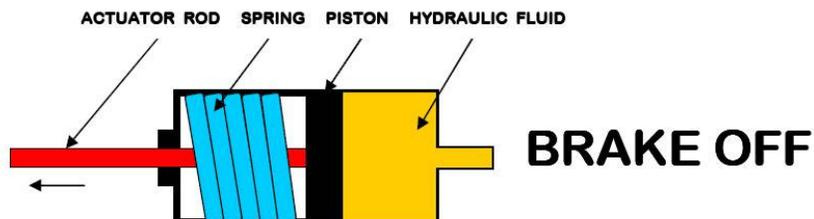
This drawing depicts the AutoPark actuator with hydraulic pressure applied. In this condition, the brake is **RELEASED**. The piston is forced to the left by the hydraulic fluid, and the actuator rod has relaxed the tension on the cable to the brake assembly.
