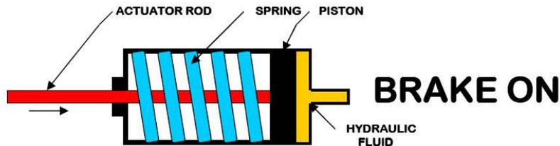
This drawing depicts the AutoPark actuator with no hydraulic pressure on it. In this condition, the brake is **APPLIED**. The piston is forced to the right by the heavy spring, and the actuator rod is putting tension on a cable connected to the brake assembly.
