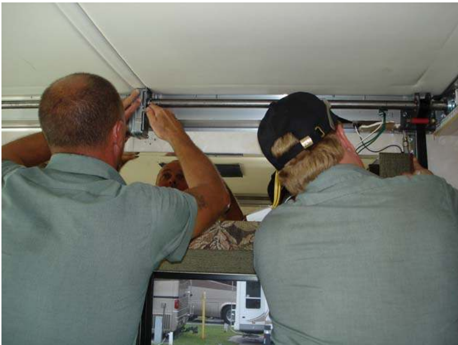
Trek Bed Curb side Reinstall Motor & Shaft
